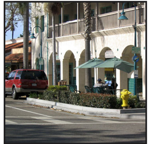
Curbside parking in Carpinteria features bulb-outs that allow sidewalk dining.
